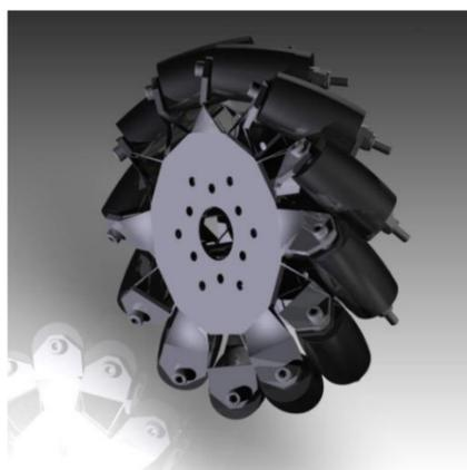
Fig 1. 3D rendering of an omnidirectional wheel
