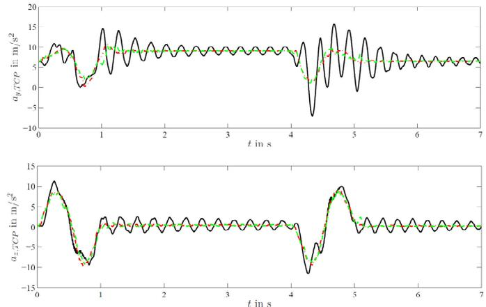
Comparison of tool center point accelerations: black: PD-motor joint-control; red: backstepping control; green: IDA-PBC
