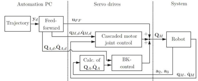
Implementation of the backstepping control (BK) using an observer calculating the arm torques  $\mathbf{Q}_A$  for the feedback loop.
