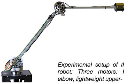
Experimental setup of the elastic articulated robot: Three motors: base, shoulder and elbow; lightweight upper- and forearm
